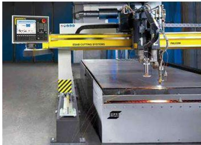
iSGM 3500 has a rugged 3-axis heavy duty gantry design for smooth motion & accuracy for improved cutting performance. With dual side, high speed AC drives and a high-speed plasma lifter, iSGM 3500 delivers higher productivity.
